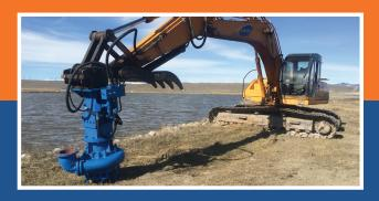
The photos depict a standard excavator with our Dredge Pump lowering the water level in the Sewage Lagoon so we can locate a pipe. This same Dredge Pump can be mounted on the Amphibious Excavators to dredge water and sludge directly from inside the lagoon or pond. A typical application would be to dredge the hard material out with the bucket and do a final clean up of the loose materials with the dredge.
